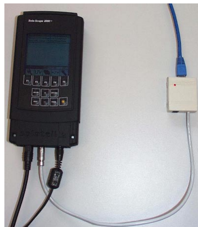
The Sola-Scope 2000 connected to the Network
