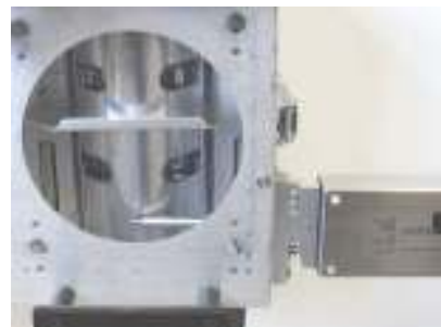
Figure 5. The probe of figure 4 in position in a microwave excited lamp's back reflector
