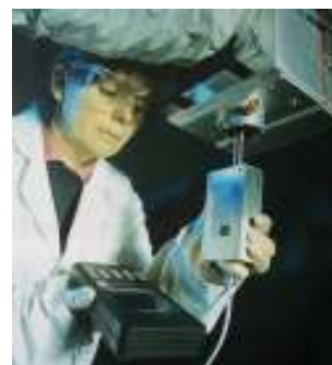
Figure 6 – measuring off-line inside quartz tube
